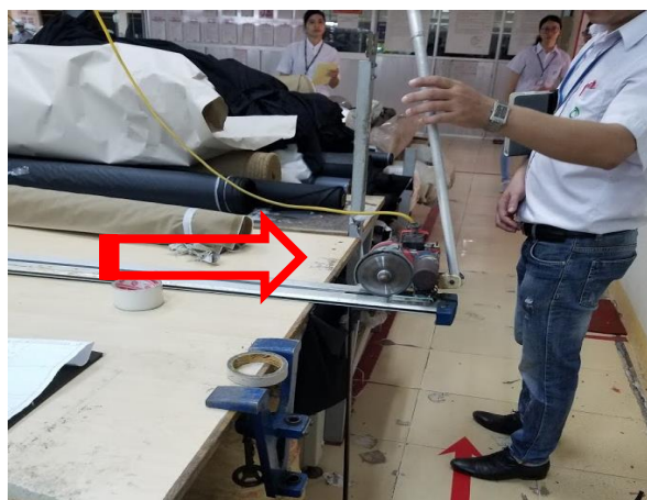
Figure 17: Unguarded Cutting Blade
