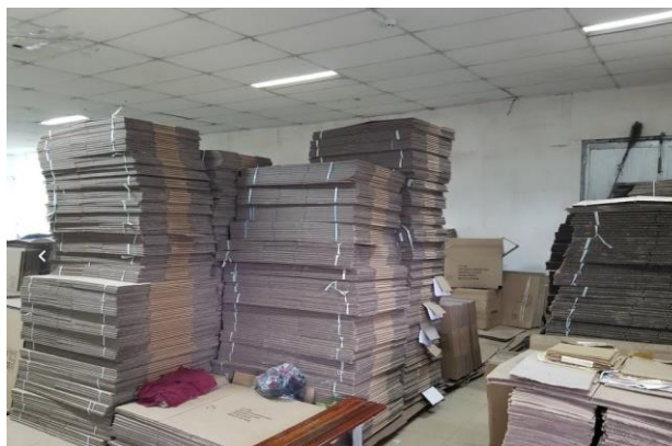
Figure 8: Excessive Storage of Combustible Packaging
