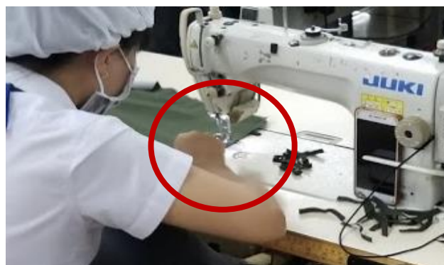
Figure 24: Lack of Guarding on Sewing Machines
