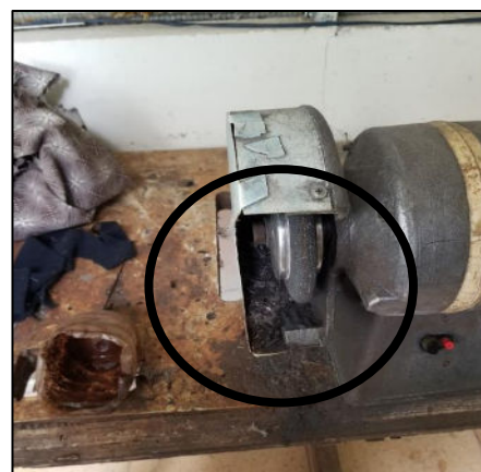
Figure 19: Unshielded Grinding Wheel
