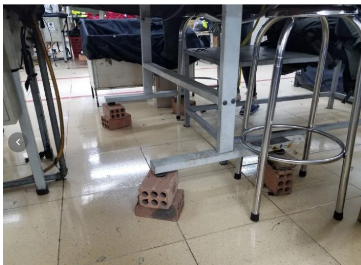
Figure 33: Worktable Propped-Up on Bricks
