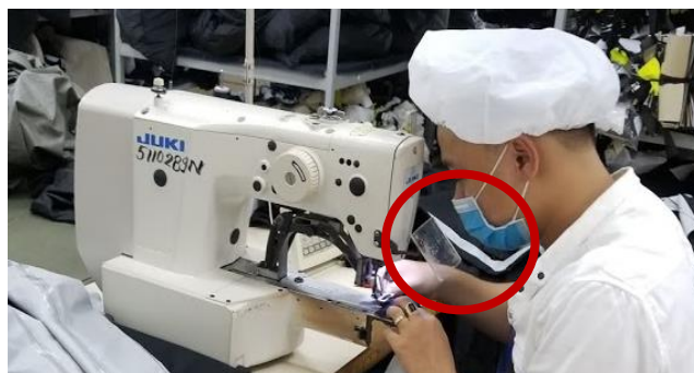
Figure 23: Sewing Machine with Guarding
