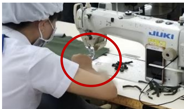
Figure 24: Lack of Guarding on Sewing Machines
