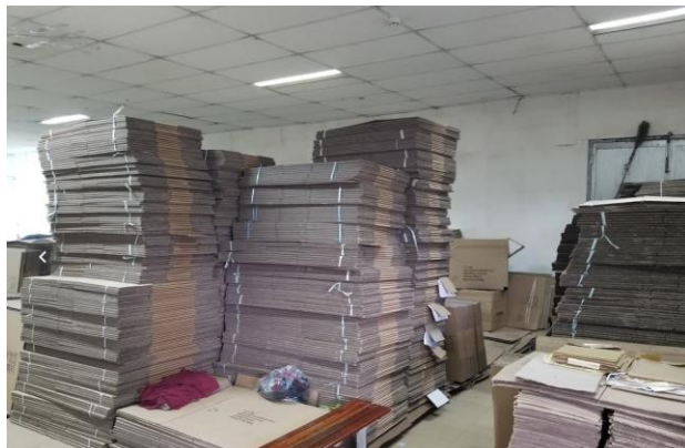
Figure 8: Excessive Storage of Combustible Packaging
