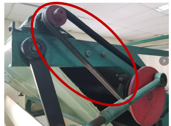
Figures 20-22: Lack of Guarding on Belt-Driven Machines
