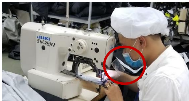
Figure 23: Sewing Machine with Guarding
