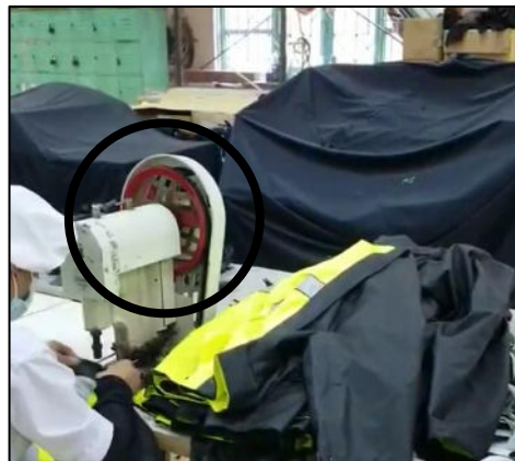
Figures 20-22: Lack of Guarding on Belt-Driven Machines
