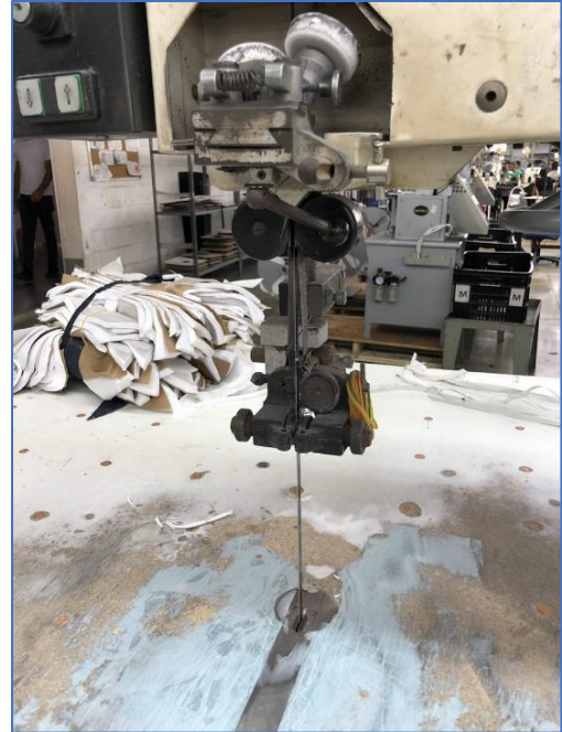
Figure 9: Fabric cutting machines missing blade guard
