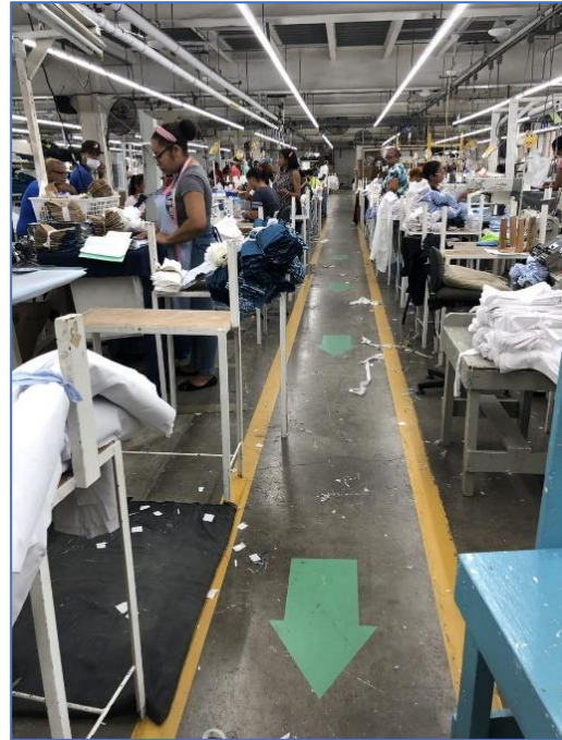
Figure 4: Partially obstructed exit path
