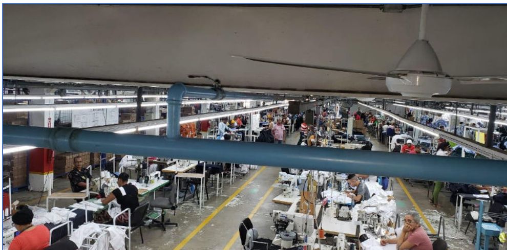
Figure 7: Dust on overhead pipes was removed. The factory has purchased four vacuum units for regular cleaning. (Figure provided by RJ Torres, August 2022)
