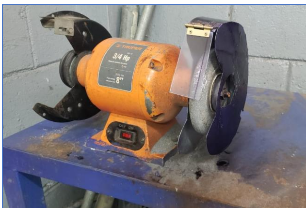
Figure 10: Tool grinder with shield protector installed. (Figure provided by RJ Torres, August 2022)
