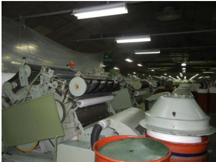
1. Carding machines with inadequate guards showing exposed belt drives. 2. Exposed belt drive on machine in batting area. 3. Unguarded roller shafts on gluer.
