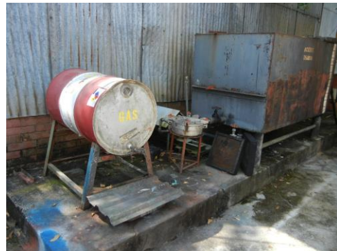
Kerosene drum without secondary containment stored outside.
