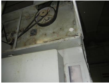
1. Carding machines with inadequate guards showing exposed belt drives. 2. Exposed belt drive on machine in batting area. 3. Unguarded roller shafts on gluer.
