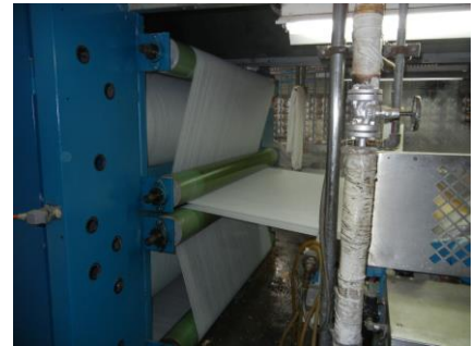
1. Carding machines with inadequate guards showing exposed belt drives. 2. Exposed belt drive on machine in batting area. 3. Unguarded roller shafts on gluer.
