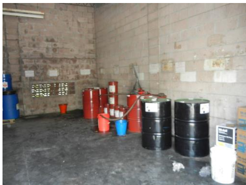
Left: Ungrounded thinner drum in flammable storage room. Note spill on floor.
