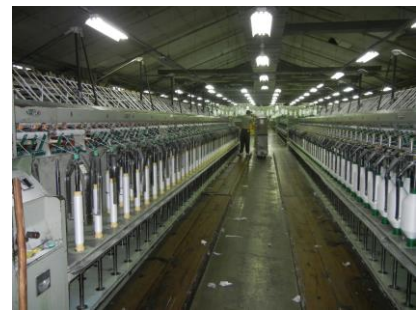
Unguarded "continuas" spinning machines with worker.
